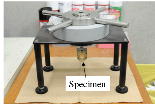
10 MPa hydrogen vessel with glass windows
