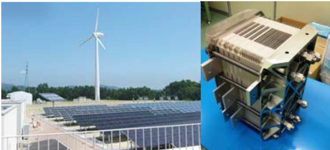
2012 Fukushima Renewable energy institute PEM type Reversible fuel cell (5.5Nm 3 /h, 2.6kW)
