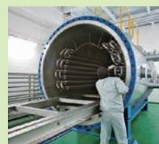
Conducting a durability test using hydrogen gas
