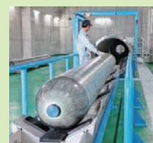
Measuring the expansion of a large hydrogen cylinder
