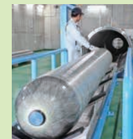
Conducting a durability test using hydrogen gas
