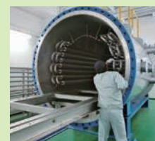
Measuring the expansion of a large hydrogen cylinder
